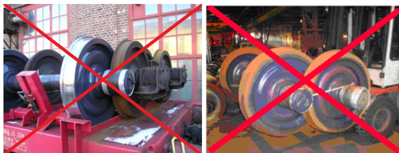
Incorrect wheelset transportation (wrong staggering)
