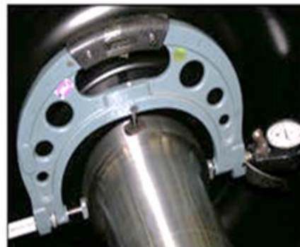
Stirrup gauge with three points used to measure D_b
