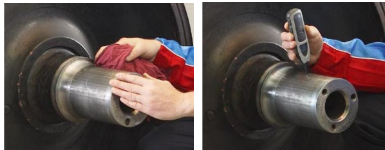
Cleaning and temperature measurement of the journal
