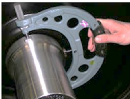
Stirrup gauge with three points used to measure D_b
